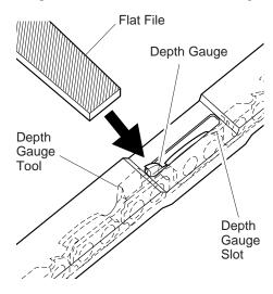
Figure 21 - Depth Gauge Tool On Chain
